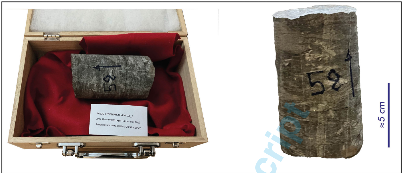
Fig. 11 - Micaschist sampled in the deep borehole Venelle (Lago area) at depth of 2900 m b.g.l., and estimated temperature of 515 °C. It was donated by ENEL Green Power Ltd. to the Department of Earth Sciences of Pisa University, November 29, 2023.
